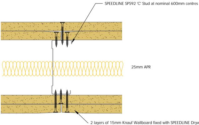
2 layers of 15mm Knauf Wallboard fixed with SPEEDLINE Drywall Screws at 300mm centres (200mm centres at external angles). Ref to table for fixing length.
